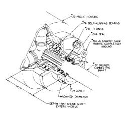
to the joint end that is on the spool adapter. This distance will not vary with misalignment since the joint is bolted and cannot move.) Put the #31A alignment gauge on the machined of the diameter #24 cover and slide it completely around. It will indicate how the engine must be moved to center the spline shaft in the oil seal. Re-measure the joints to see if
