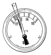
7. As soon as the engine has started, release both Start and Preheat buttons. Check that with engine running, oil pressure and battery charge voltage are registering and that raw water is discharging with the exhaust.
