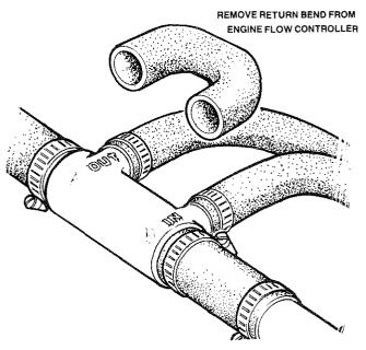
Model W 46 comes complete with a Flow Control which, when properly connected to a heater tank, produces domestic hot water from waste engine heat.
