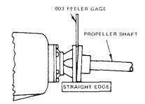
CHECKING COUPLING ALIGNMENT
